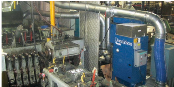
WSO on Smoke - Cold Forming 1,200 cfm (2,038 m 3 /h)
