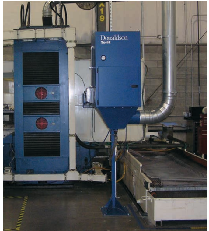
WSO on Water Mist - Horizontal Grinder 850 cfm (1,444 m 3 /h)
