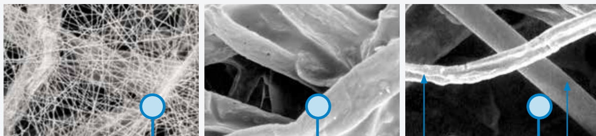
10 Micron Nanofiber Technology (600x)
